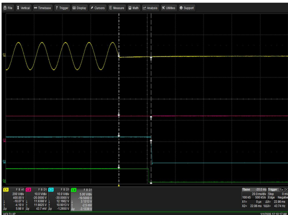
Figure 15: CSU2000AP-3-111 Hold-Up Time Vin = 90Vac Load: I O = 102.5A I SB = 3.5A Ch 1: AC Mains Ch 2: V SW Ch 3: V O Ch 4: PWOK
