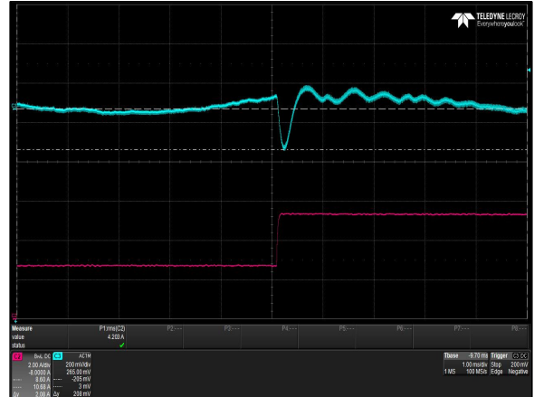
Figure 29: CPS258-M Transient Response - Vo Deviation Vin = 115 Vac Load: Io = 50% to 100% load change, 1 A/us Ch 2: Io Ch 3: Vo
