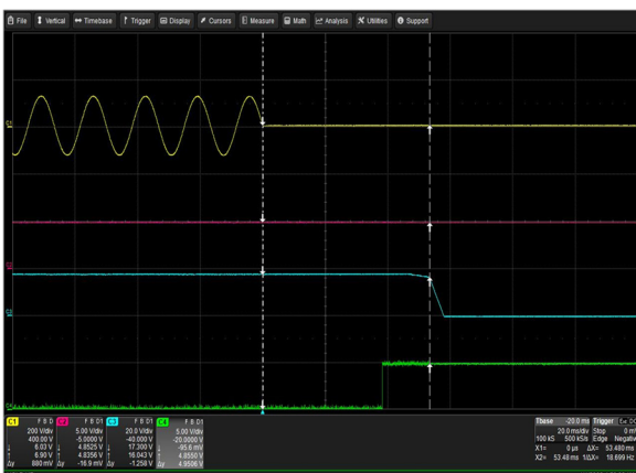
Figure 19: LCM30008-T Hold-up Time Vin = 90Vac Load: lo = 83.3A (18V), Isb = 2A Ch 1: Vin Ch 2: Vsb Ch 3: Vo Ch 4: G_DCOK_C
