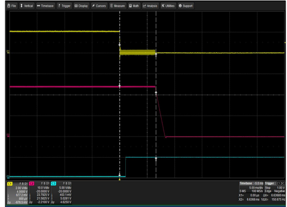
Figure 36: LCM3000Q-T Turn Off Characteristic via INH_EN Vin = 264Vac Load: Io = 125A (24V), Isb = 2A Ch 1: INH_EN Ch 2: Vo Ch 3: G_DCOK_C
