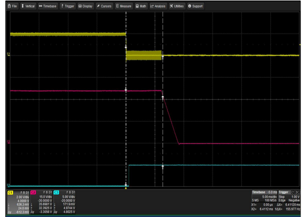
Figure 50: LCM3000U-T Turn Off Characteristic via INH_EN Vin = 264Vac Load: Io = 83.3A (36V), Isb = 2A Ch 1: INH_EN Ch 2: Vo Ch 3: G_DCOK_C
