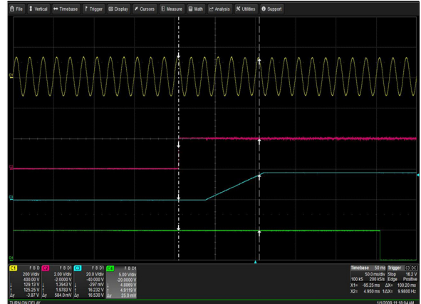
Figure 16: LCM30008-T Turn-on delay via INH_EN Vin = 90Vac Load: lo = 83.3A (18V), Isb = 2A Ch 1: Vin Ch 2: INH_EN Ch 3: Vo Ch 4: G_DCOK_C
