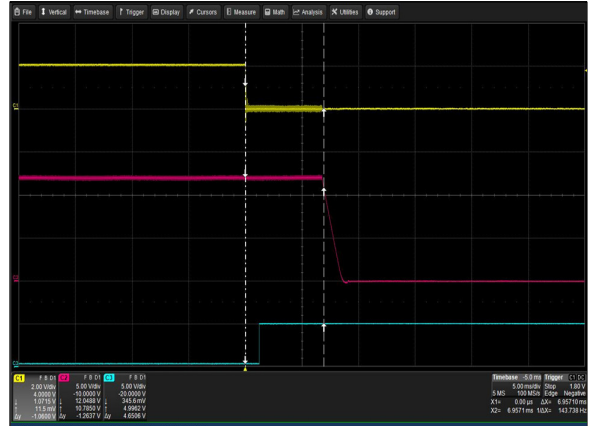
Figure 8: LCM3000L-T Turn Off Characteristic via INH_EN Vin = 264Vac Load: Io = 125A (12V), Isb = 2A Ch 1: INH_EN Ch 2: Vo Ch 3: G_DCOK_C
